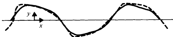
FIGURE 4. The dashed line represents the observed centre-line of the reach of the Beaver River in figure 3a; the solid line represents the approximation provided by equation (5) with \delta = 0.98 , J_F = 0.073 and J_S = 0.103 .
